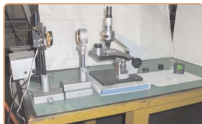
Photo of an experimental model of the reflective conoscope, developed in cooperation by IMT-Bucharest and S.C. ProOptica S.A.
