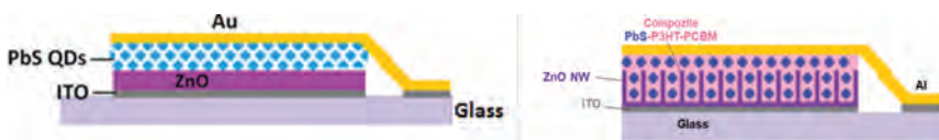
ZnO-PbS QDs heterojunction based photodetectors (left), ZnO NW- PbS QDs:P3HT:PCBM ternary blend photodetector (right)
