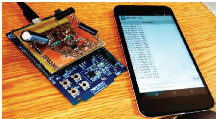
Fig 12 – Resistive measurements using the sensor device
