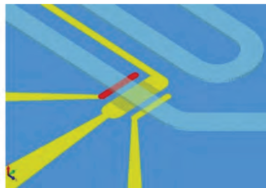
Detail in the region of an impedimetric sensor with interdigitated electrodes
