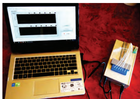
Fig. 1 The BioSIM platform: 1. Fluidic module and sensors package; 2. Electronic module; 3. Data acquisition system
