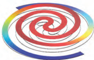
Fig. 9 Spiralled structure with 4 spires, designed for resonant frequencies in the 90 Hz range
