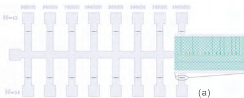
(a) Image of the designed \text{MoS}_2 -based SSDs for mask fabrication (via CleWin software);
