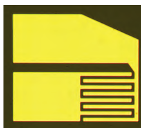
Optical images of fabricated interdigitated structures: digit / interdigit width -10 \mu\text{m}
